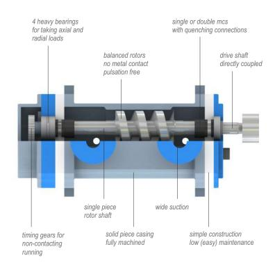
The BoMax ePDP NL-series positive displacement pumps have been entirely developed in The Netherlands, where they are manufactured in accordance with the highest quality standards.
