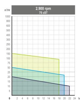
Performance curves of the BoMax ePDP NL-series, powered by 1.480 rpm and 2.900 rpm electric motors, based on processing fluids with a viscosity of 75 cSt.
